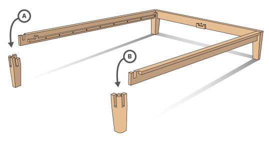
Place the remaining Short Rail into the Legs, "U" joint facing down, and press it down fully.
