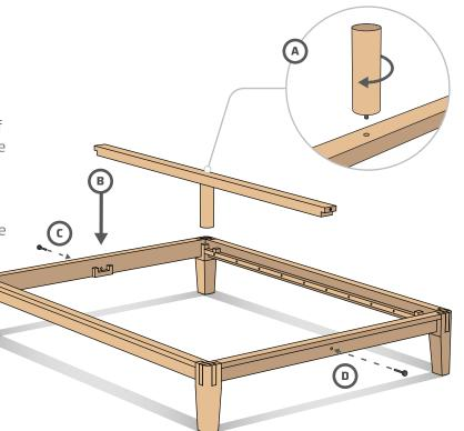
A. Lay rolled Slats down at the head of The Bed. Place the first slat between the Short Rail and Slat Stop to hold in place.
